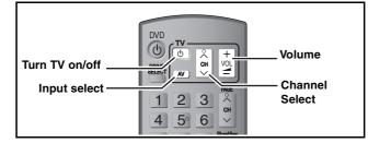
Point the remote control at the television While pressing [<sup>(1)</sup> TV], enter the code with the numbered buttons. e.g., 01: [0] → [1] 10: [1] → [0]
